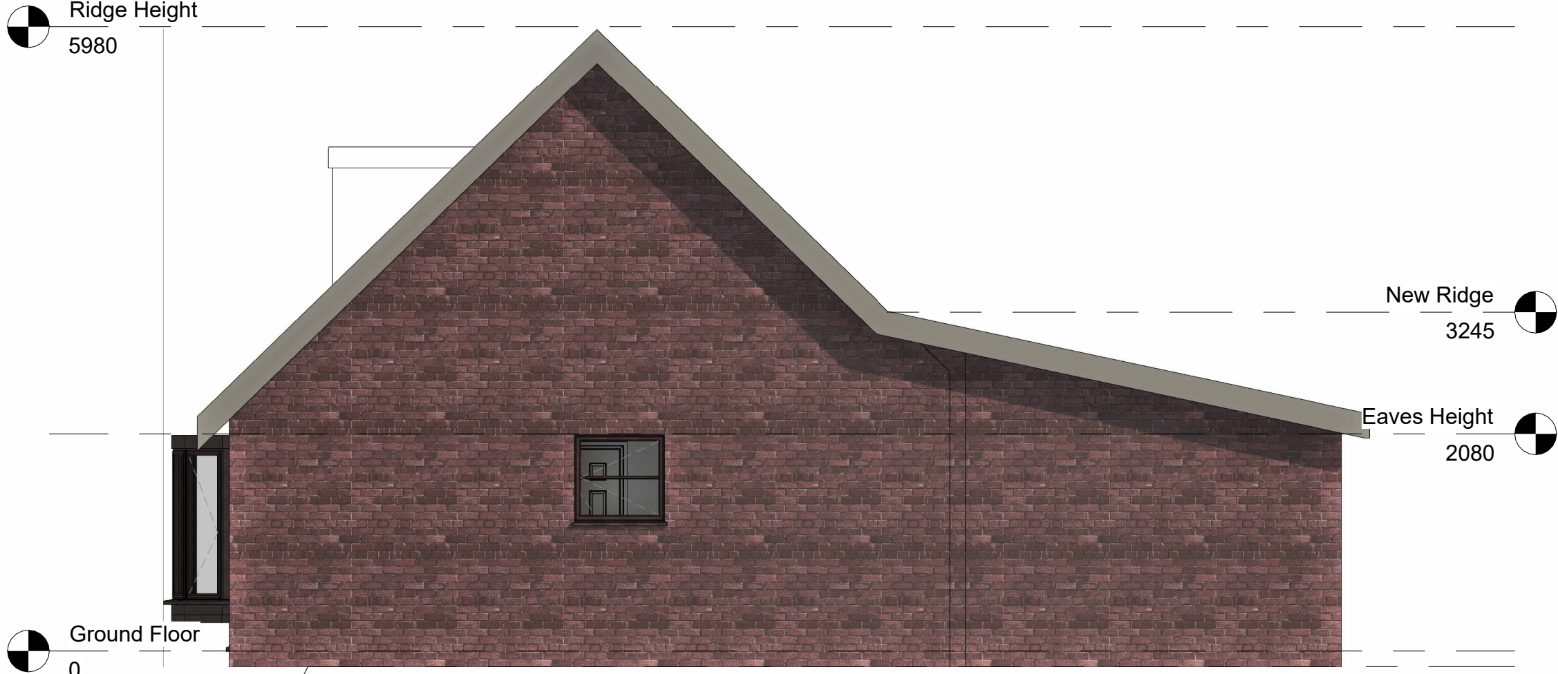
4 Proposed RHS Gable Elevation 1 : 50
