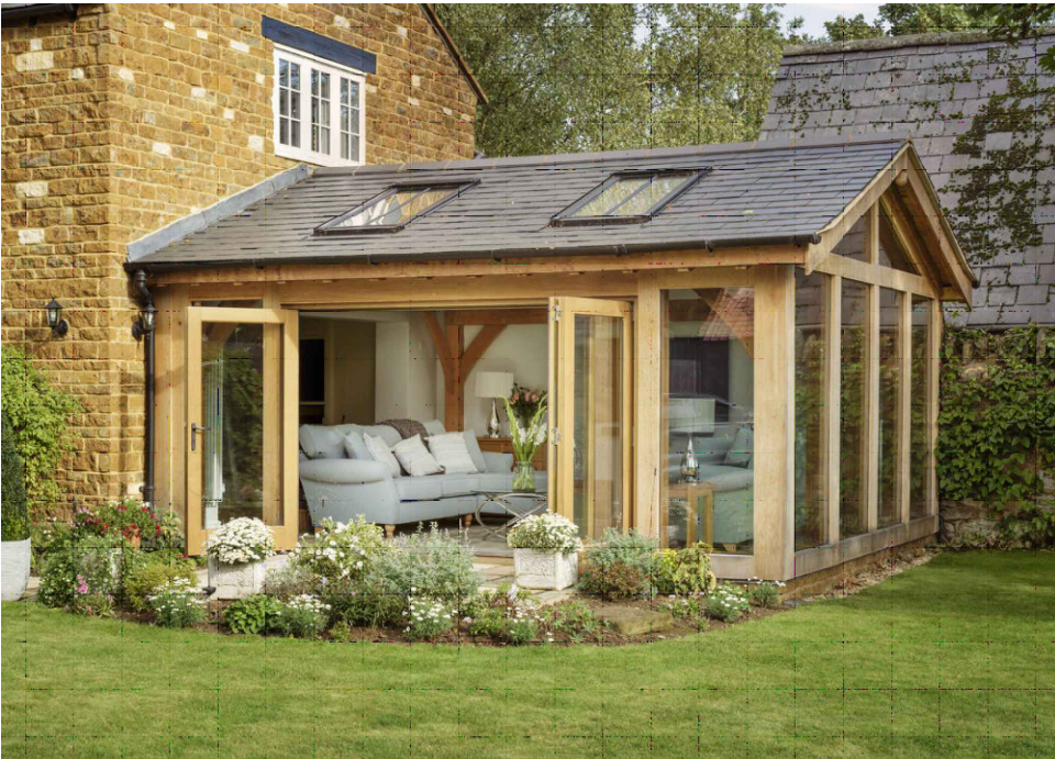
EXAMPLE OAK FRAMED GLAZED OPENINGS AND STRUCTURE
