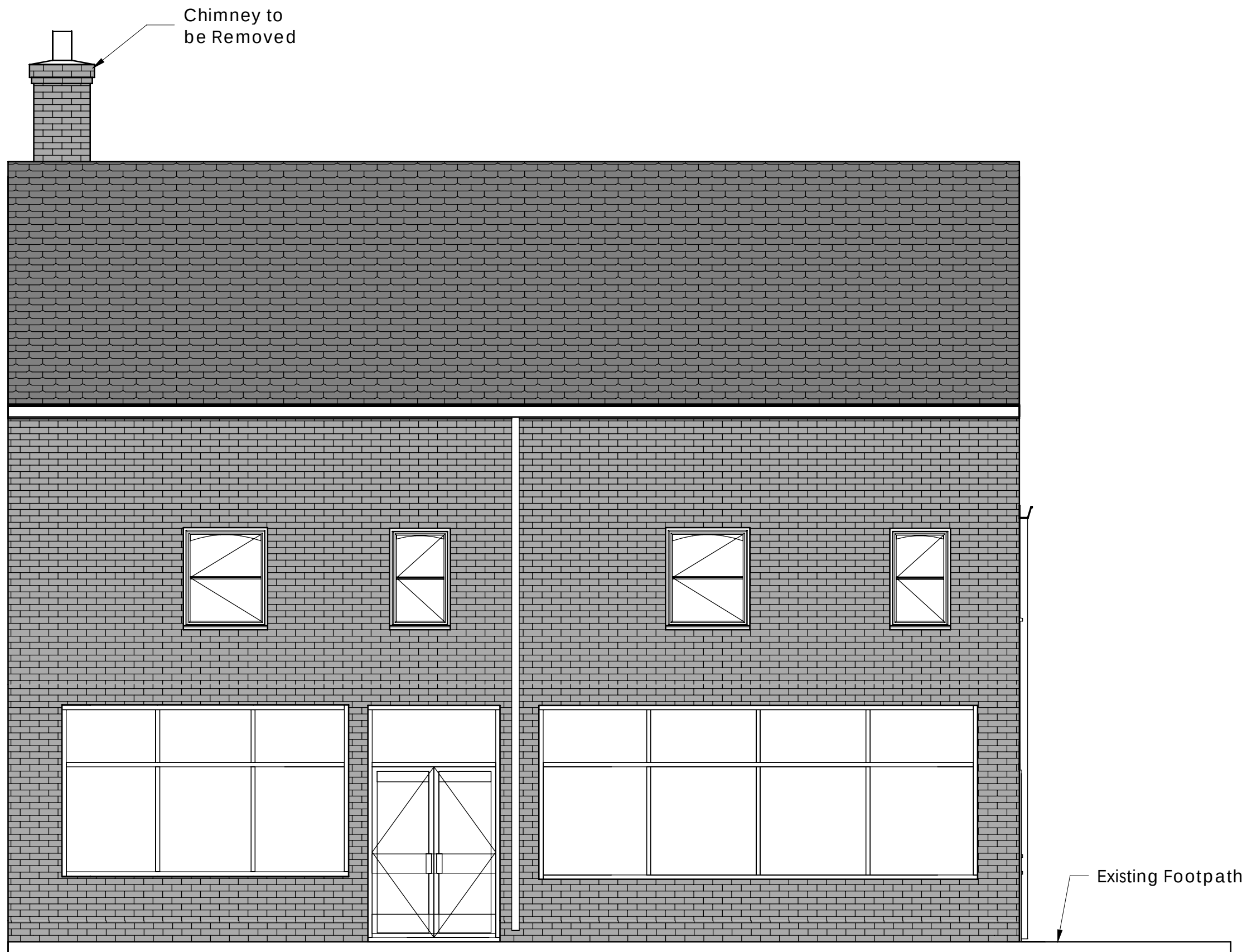
1 Existing Front Elevation 1 : 50
