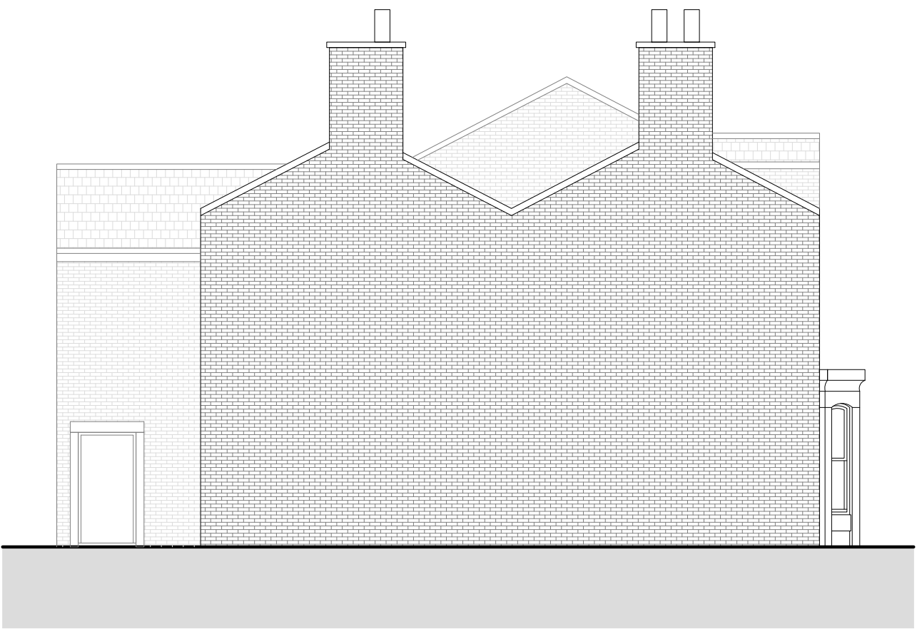
EXISTING SIDE ELEVATION 1:100 @ A1
