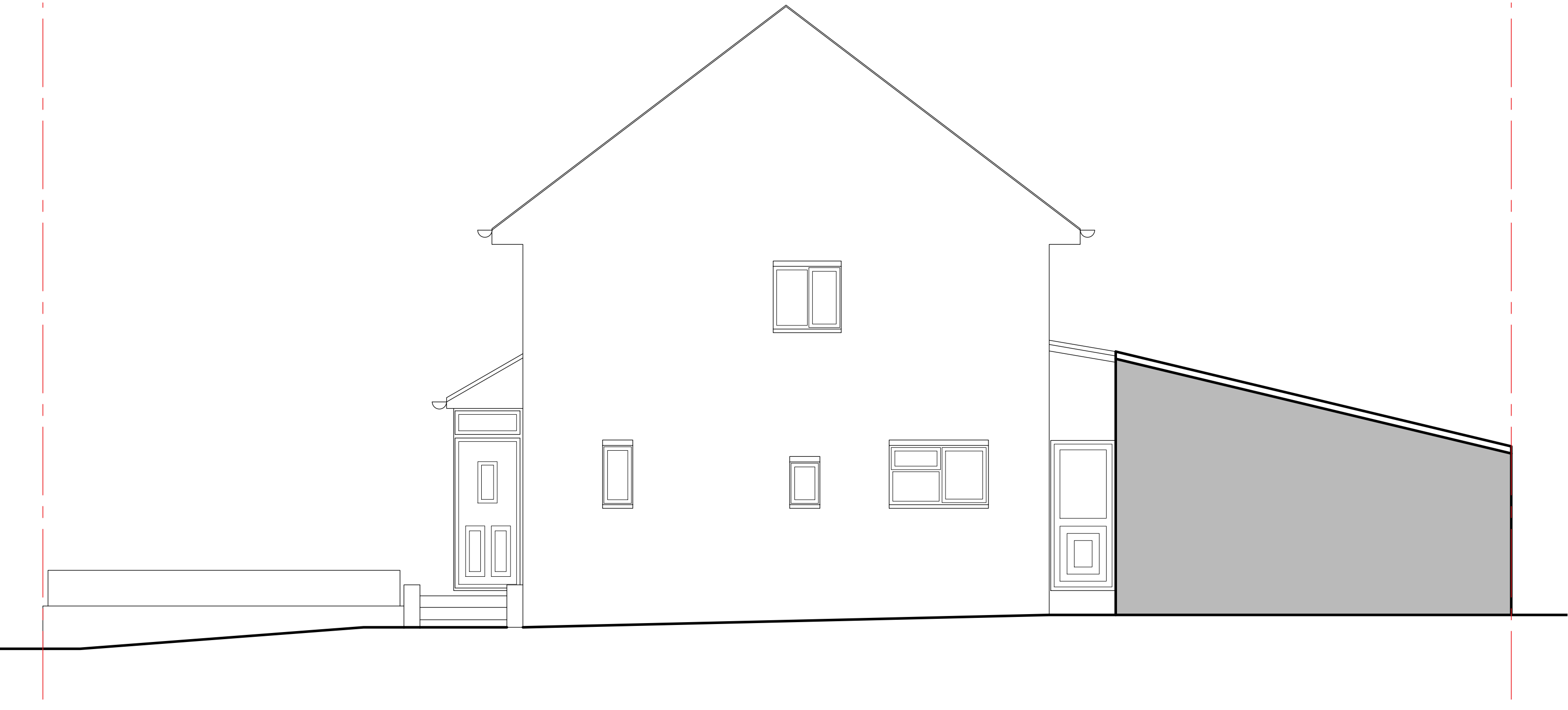
Existing Gable 2 Elevation scale 1:50
