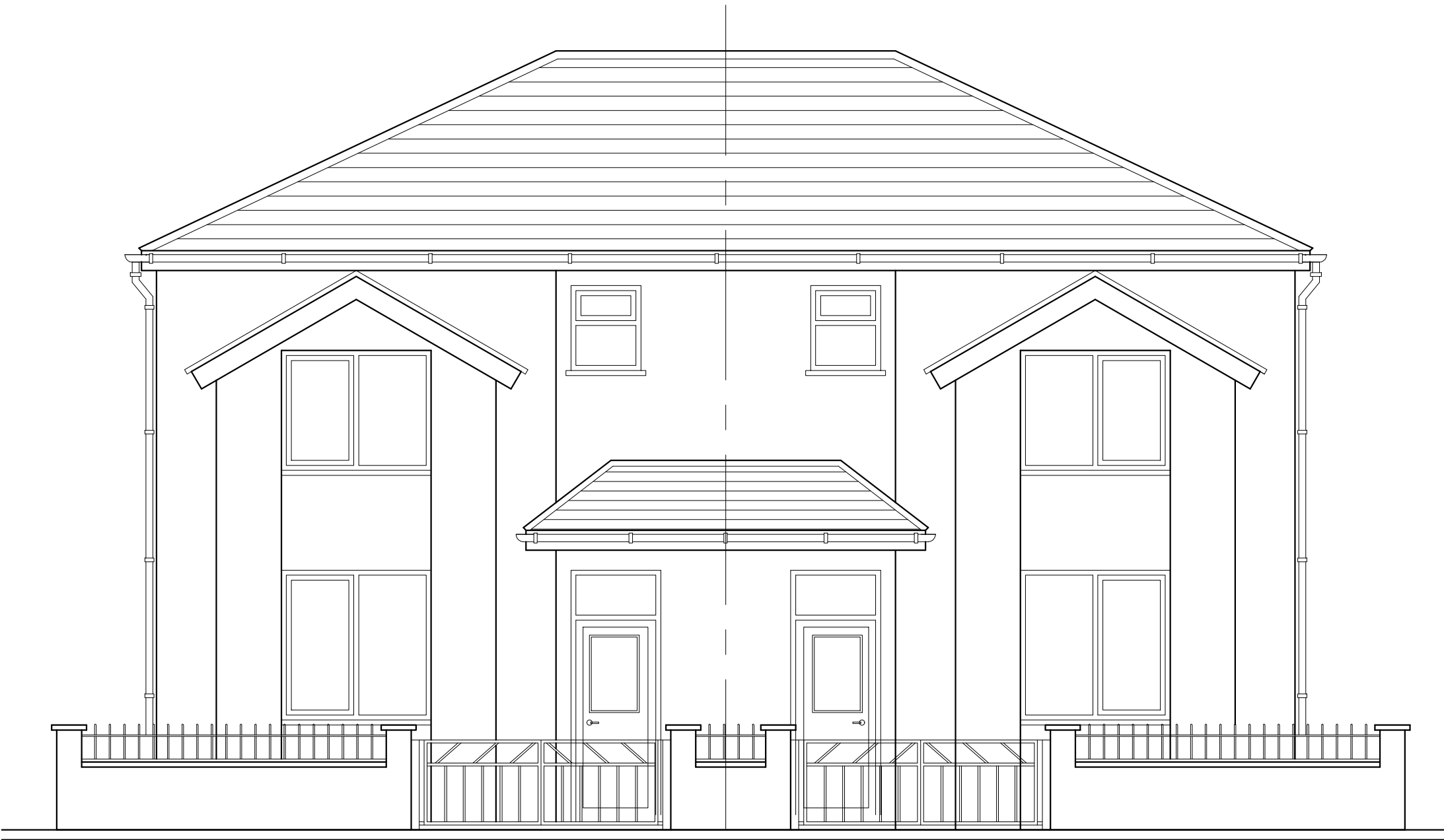
FRONT ELEVATION WITH BOUNDARY WALL
