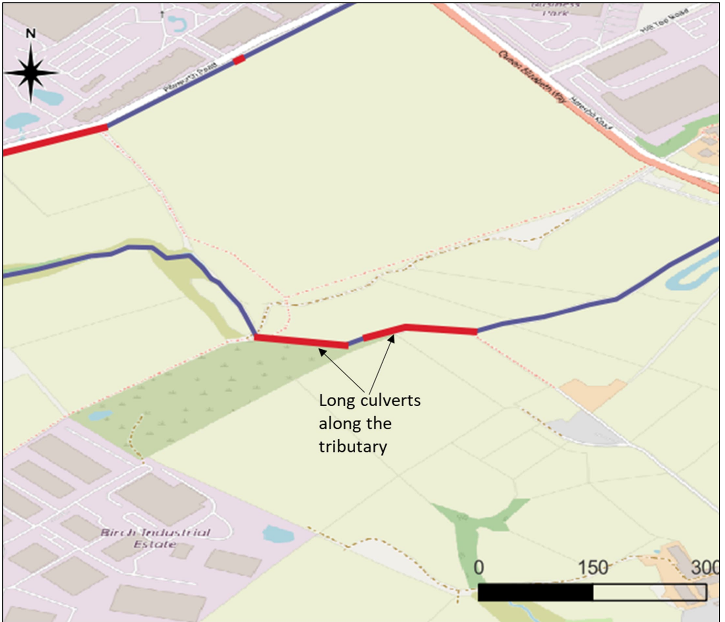
Figure 6 - Long culvert along tributary
