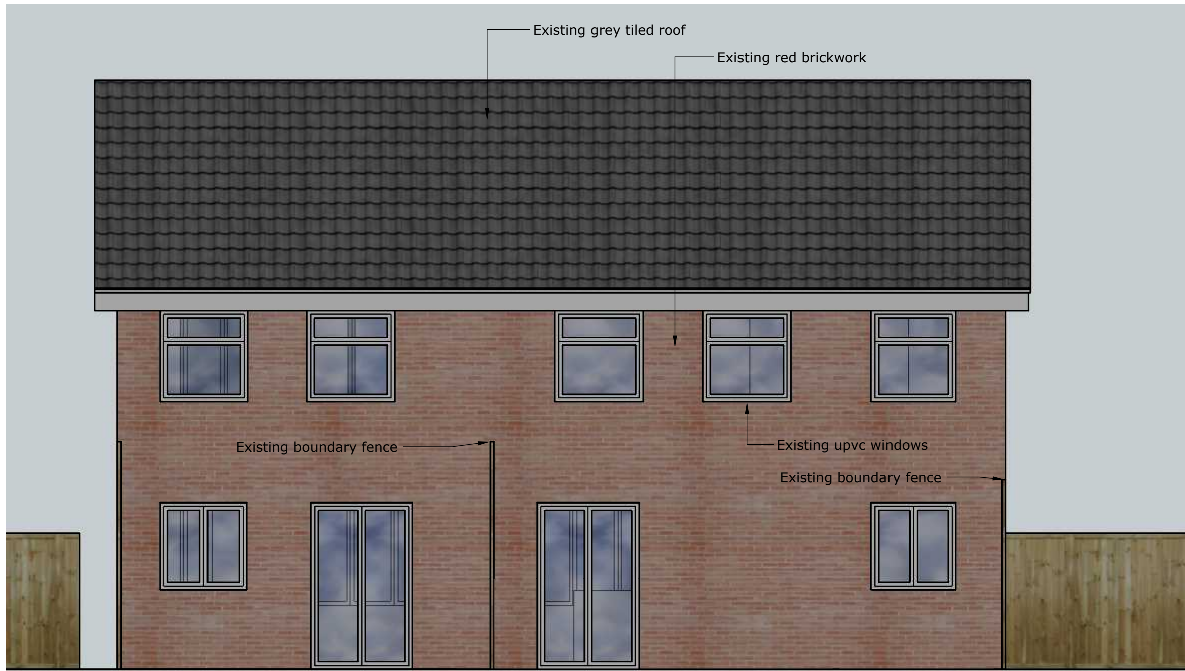
1 Existing South West Elevation Scale: 1:50
