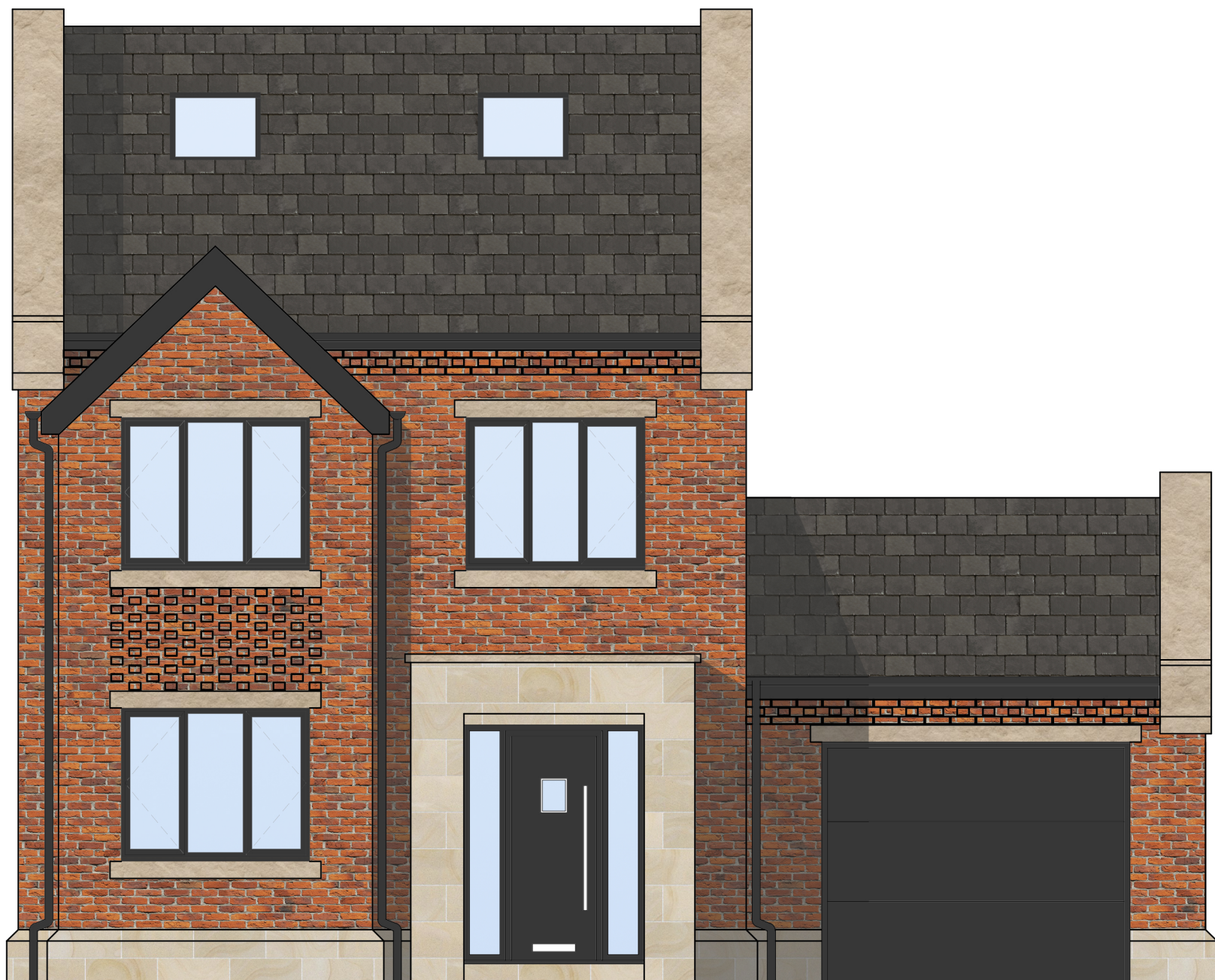
PLOT 1 & 2 FRONT ELEVATION AS PROPOSED (1:50)
