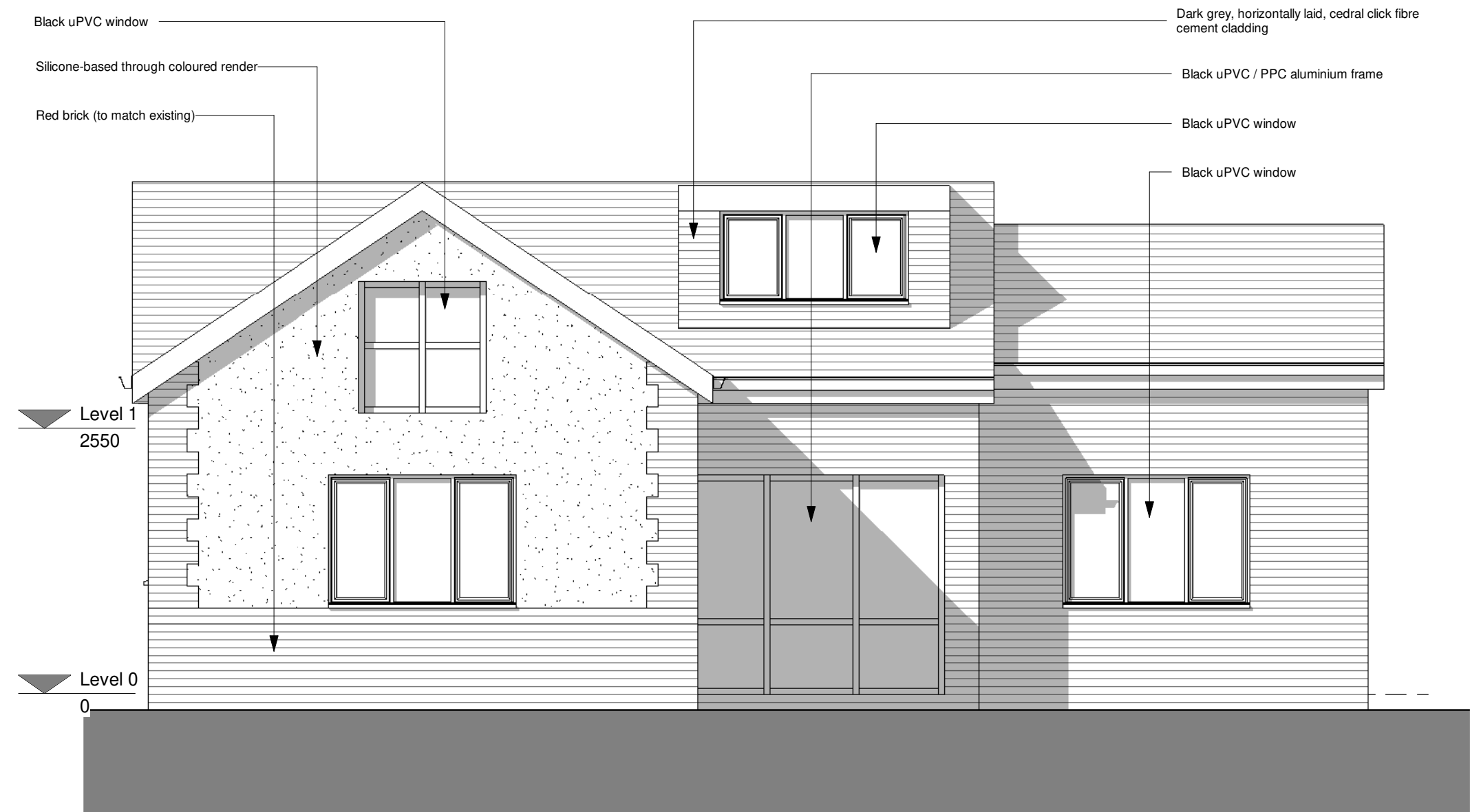
Proposed South Elevation 1 : 50
