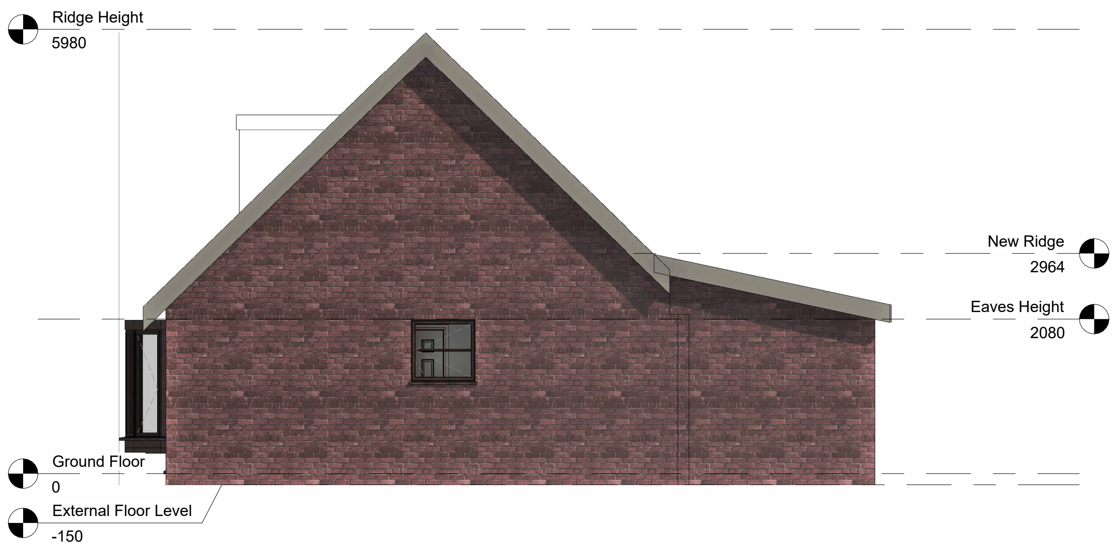
4 Proposed RHS Gable Elevation 1 : 50
