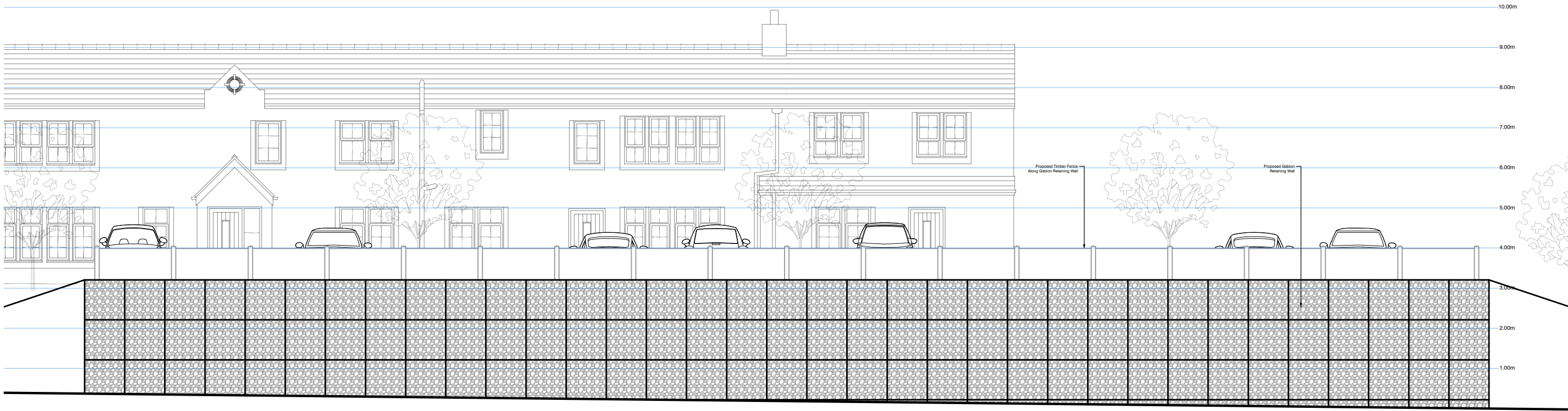
PROPOSED RETAINING WALL ELEVATION SCALE: 1:100
