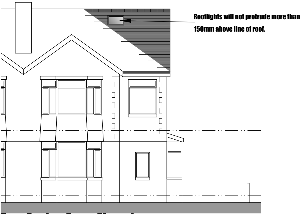
East Facing Front Elevation
