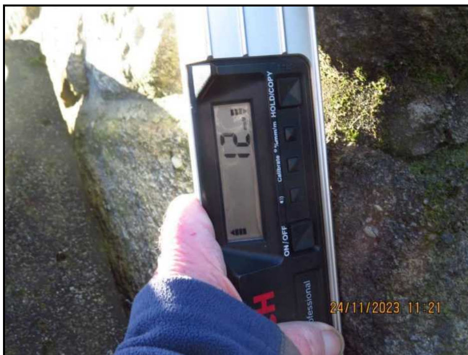
009 Vertical alignment \pm 6mm per metre
