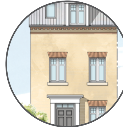
Flat Arch Brick Lintels to first floor Windows (Greenwood)
