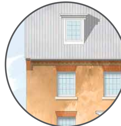
Dentilled Eaves Brickwork and Corbals (Emerson)
