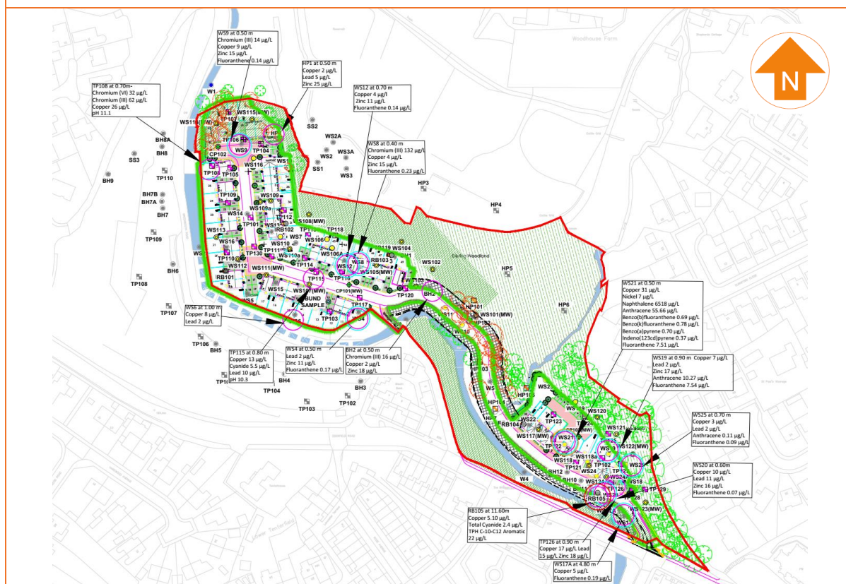
FIGURE 4.10 CONTAMINATION ISSUES PLAN – LEACHATE
