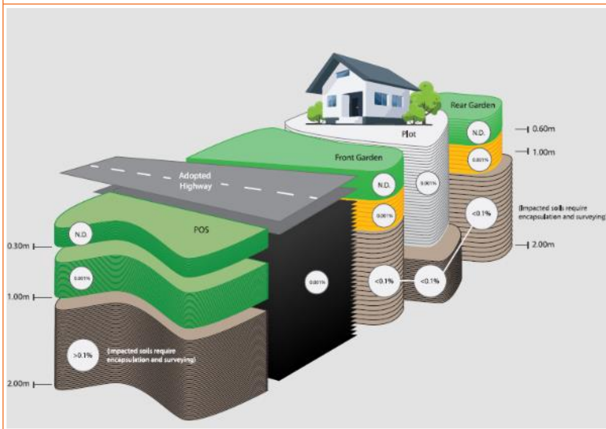
FIGURE 4.8 ASBESTOS RISK MITIGATION CONCEPTUAL SITE MODEL
