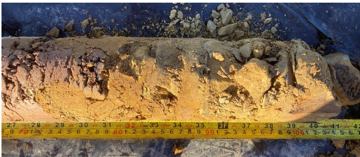
Figure 7-C: Weathered Pennine Lower Coal Measures Formation deposits in WS05
