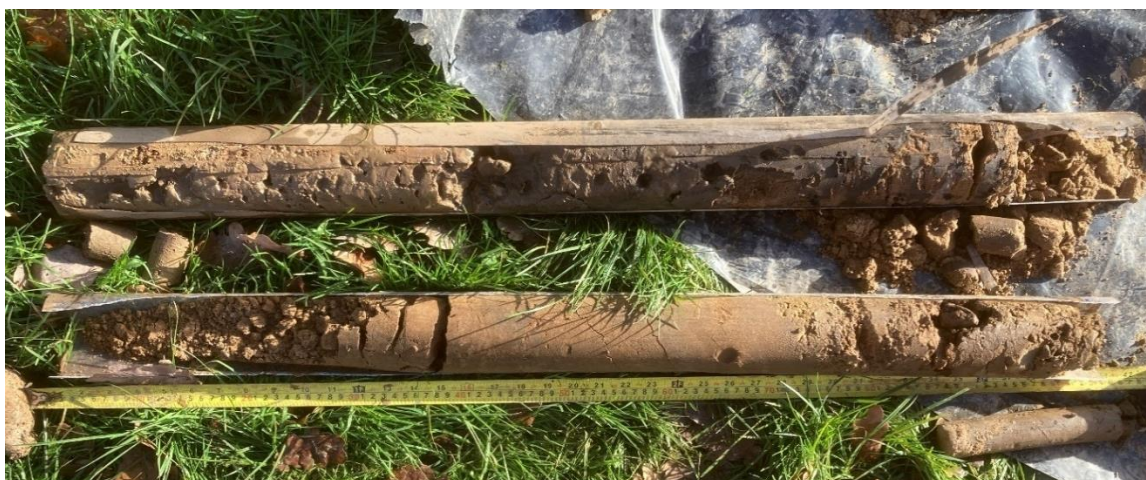
Figure 7-B: Devensian Till deposits taken from WS04
