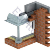
Corner Window Lintel Detail
