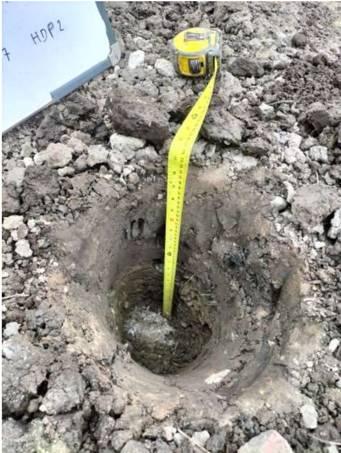
Topsoil and sub-soil layers within HDP2, Plot 7. Geotextile visible at the base.
