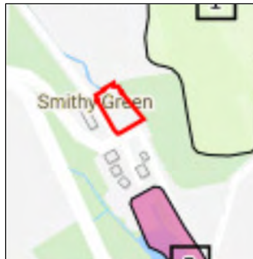
Figure 11: Extract showing the location of the infilled ground (light green) and worked ground (pink)
