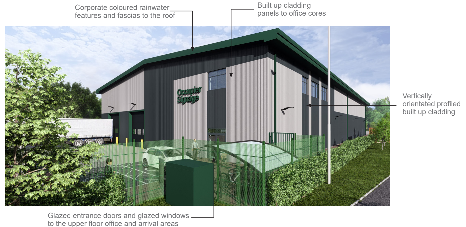
Above: Corporate coloured cladding will be used to highlight architectural features along the elevations
