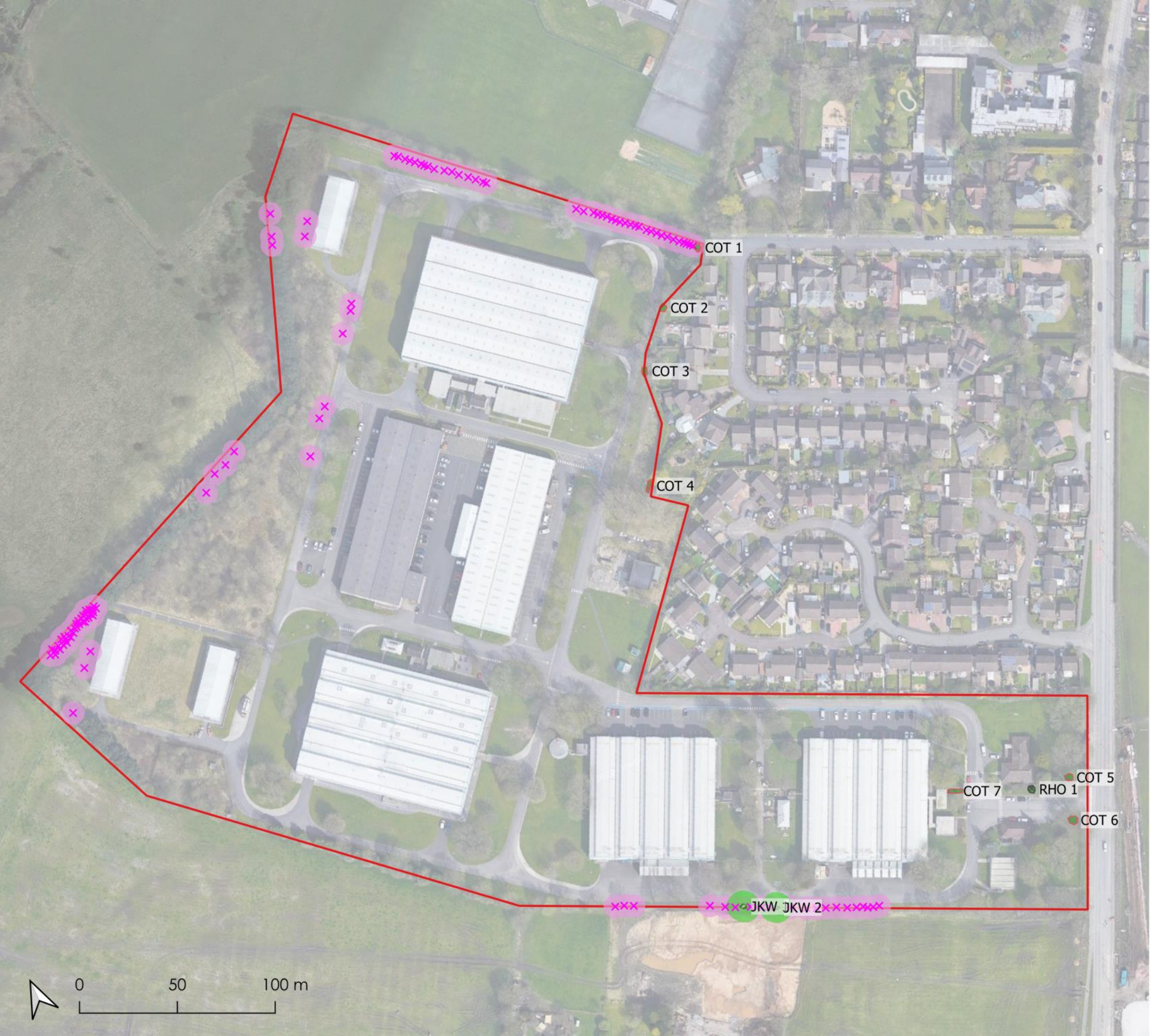
Figure 4 Whole site: Buffers to JKW (7m) and HB (6m) to show potential spread into surrounding soils, in relation to aerial photography
