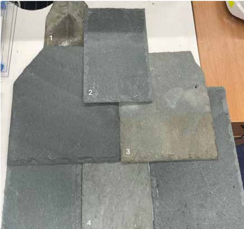
4.2 Comparison of the Different Roof Slates. Clockwise From Top Left. 1) Reclaimed Westmorland 2) Riven Westmorland 3) Existing Slates 4) Vermont Slates
