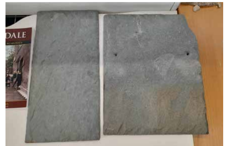
4.6 Proposed Vermont Slate (L) adjacent to Existing Westmorland Slate (R)
