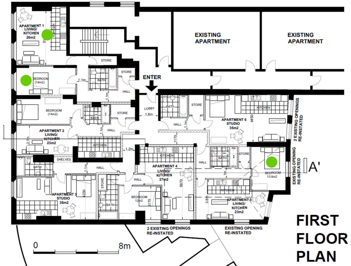
Figure 10 – Internal Layout Ground and First Floor
