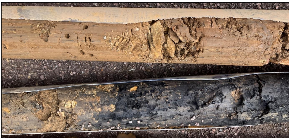
Figure 5-B: Made Ground – Reworked Till encountered within WS02
