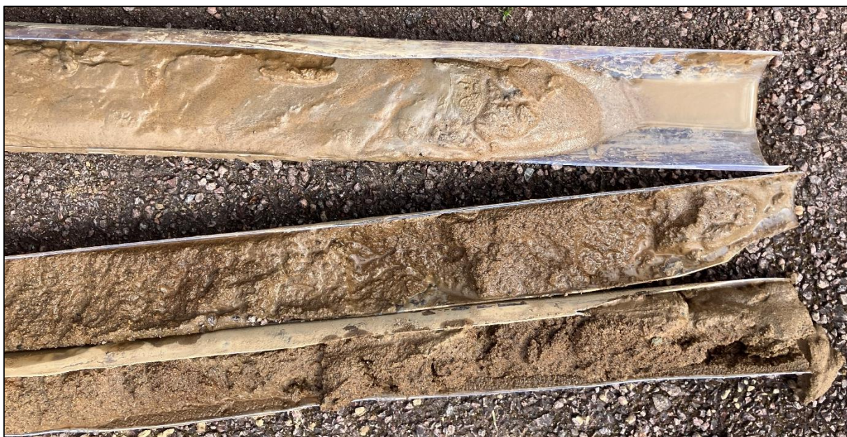
Figure 5-C: Glaciofluvial Deposits encountered within WS02
