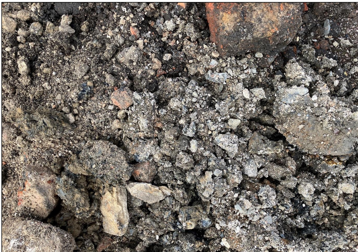
Figure 5-A: Made Ground encountered within WS01
