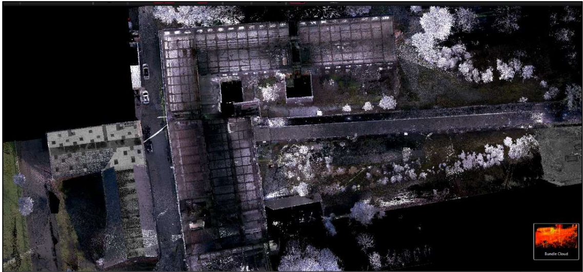
Plate 18: Second floor plan of Marina Ropeworks taken from the 3D digital point cloud
