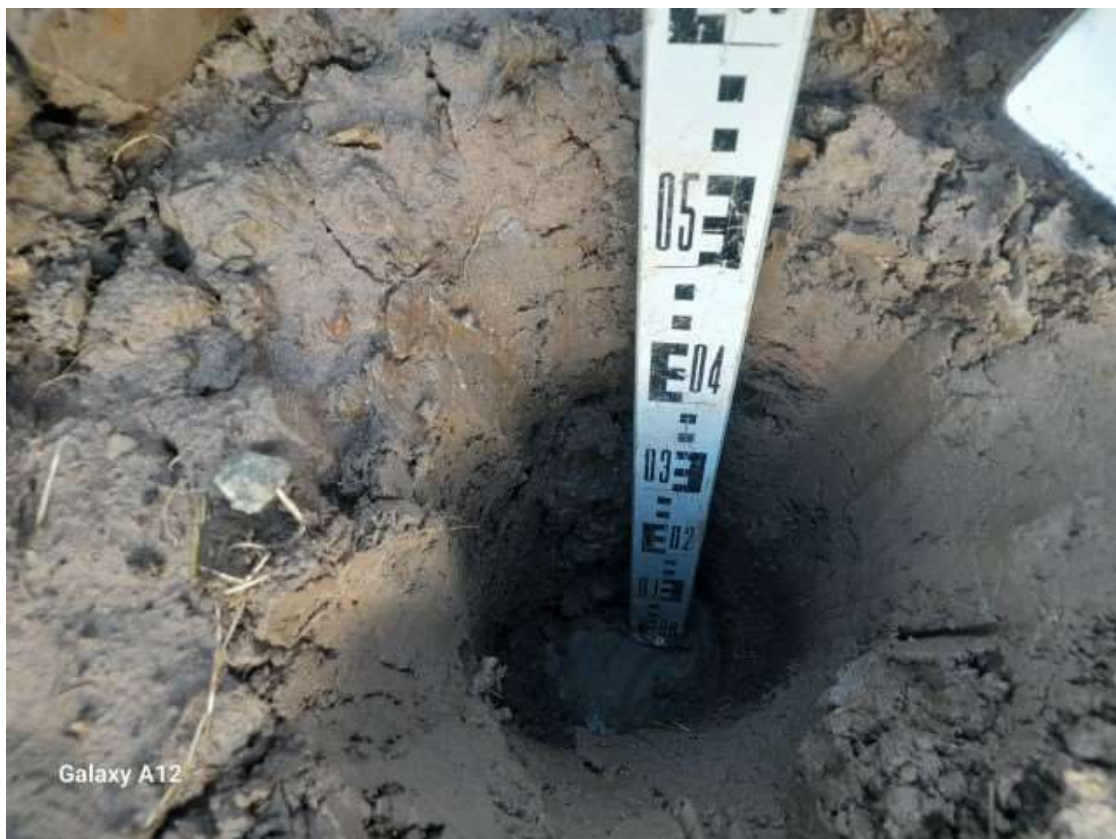
Geotextile membrane at the base of hand dug pit HDP1.
