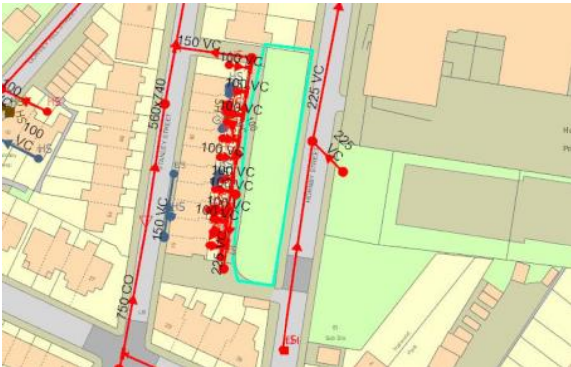
Figure 3: UU Sewer record extract
