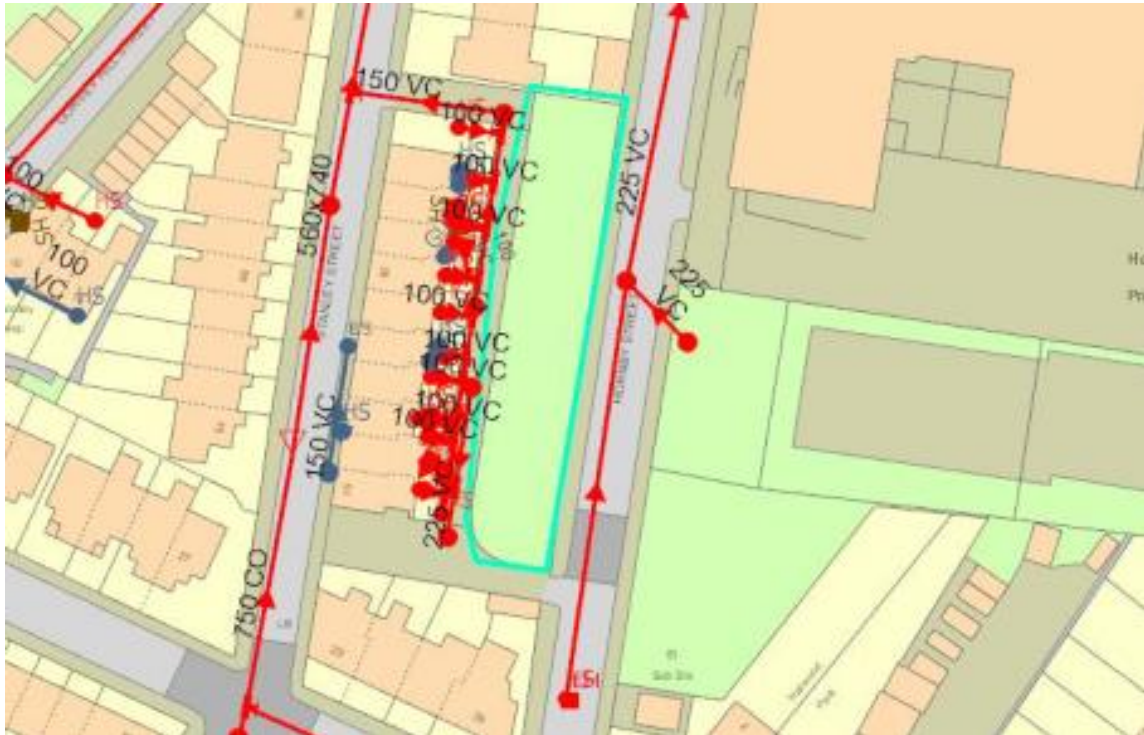
Figure 3: UU Sewer record extract
