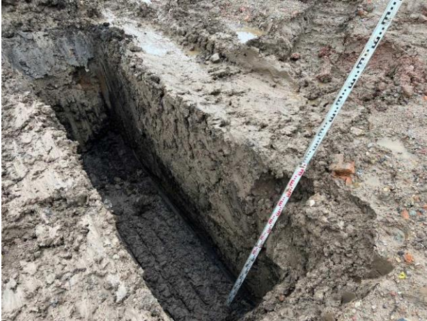
Photograph 104 (left) & 105 (right): A view of photograph 104, showing the peat deposits still present on the eastern face of Trial pit TP404 in front of Plot 141. Similarly, photograph 105 shows peat deposits present on the western face of the trial pit in front of Plots 136-138, dated 20 th March 2023.
