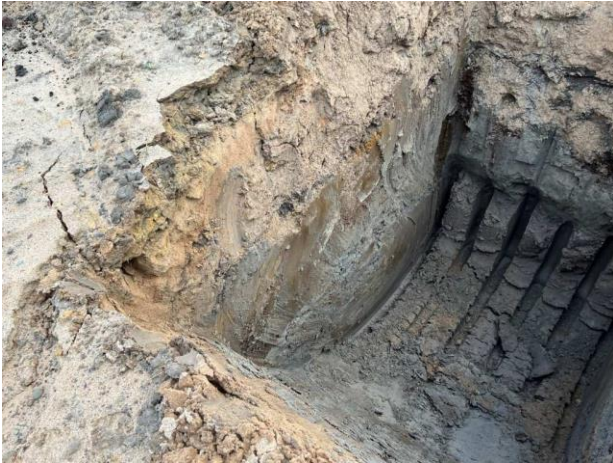
Photograph 102 (left) & 103 (right): A view of photograph 102, showing the eastern face (right field of view) of the small excavation in the rear garden of Plot 142 exposing a thin band of peat, with no peat present toward the western edge of the excavation. In a similar vein, photograph 103 shows intermittent peat deposits present in the southern face of the excavation in the rear garden of Plots 139-140, with the peat thinning toward the western extreme of the excavation, dated 27 th October 2022.
