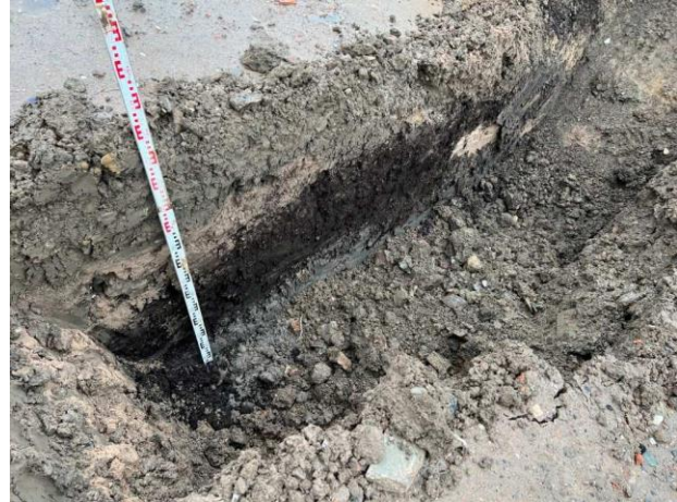
Photograph 104 (left) & 105 (right): A view of photograph 104, showing the peat deposits still present on the eastern face of Trial pit TP404 in front of Plot 141. Similarly, photograph 105 shows peat deposits present on the western face of the trial pit in front of Plots 136-138, dated 20 th March 2023.
