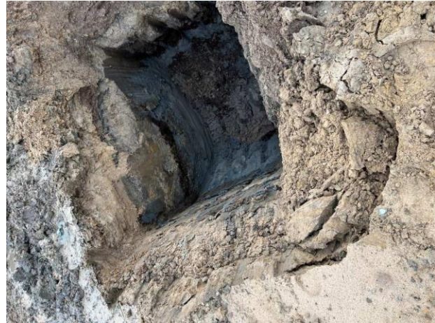
Photograph 102 (left) & 103 (right): A view of photograph 102, showing the eastern face (right field of view) of the small excavation in the rear garden of Plot 142 exposing a thin band of peat, with no peat present toward the western edge of the excavation. In a similar vein, photograph 103 shows intermittent peat deposits present in the southern face of the excavation in the rear garden of Plots 139-140, with the peat thinning toward the western extreme of the excavation, dated 27 th October 2022.
