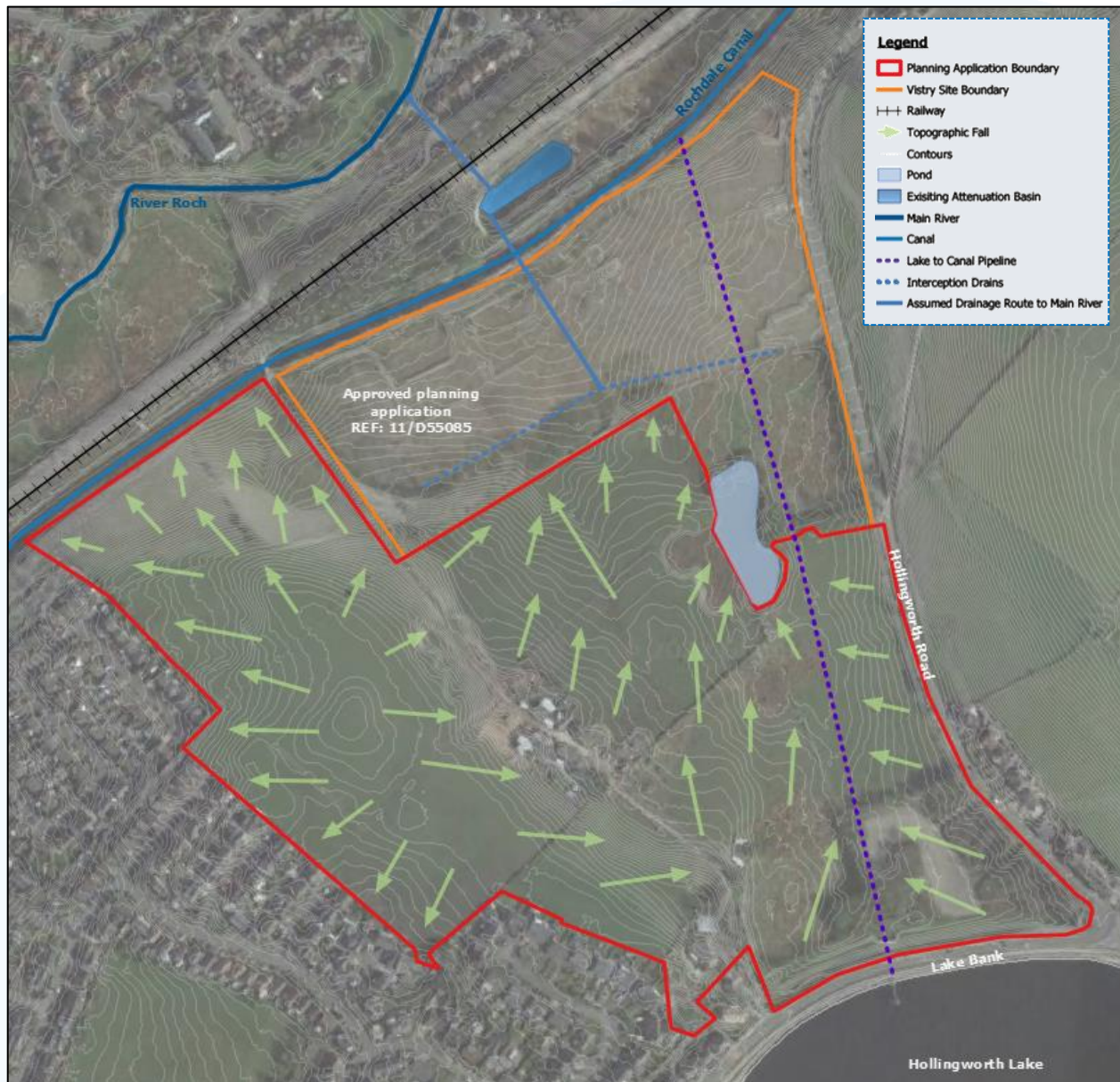
Figure 3: Existing Drainage Plan (Betts Hydro, 2022)
