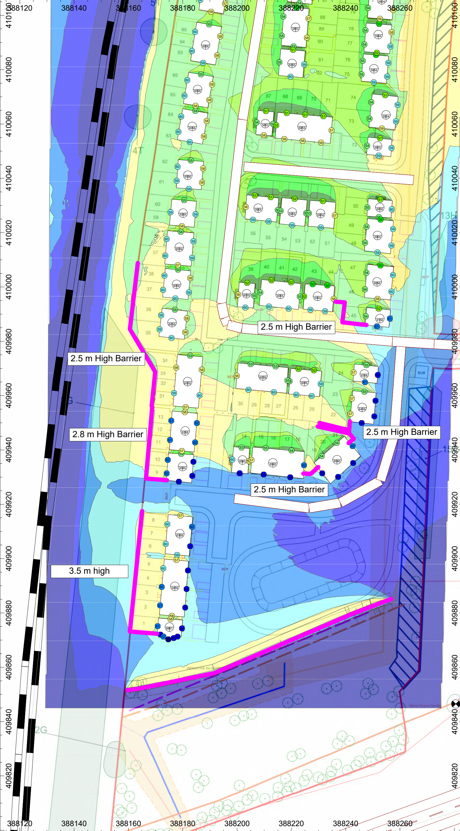
Figure 7 - Daytime with Mitigation Grid Noise Map (BS 8233) - Calculation at 1.5 m above ground level
