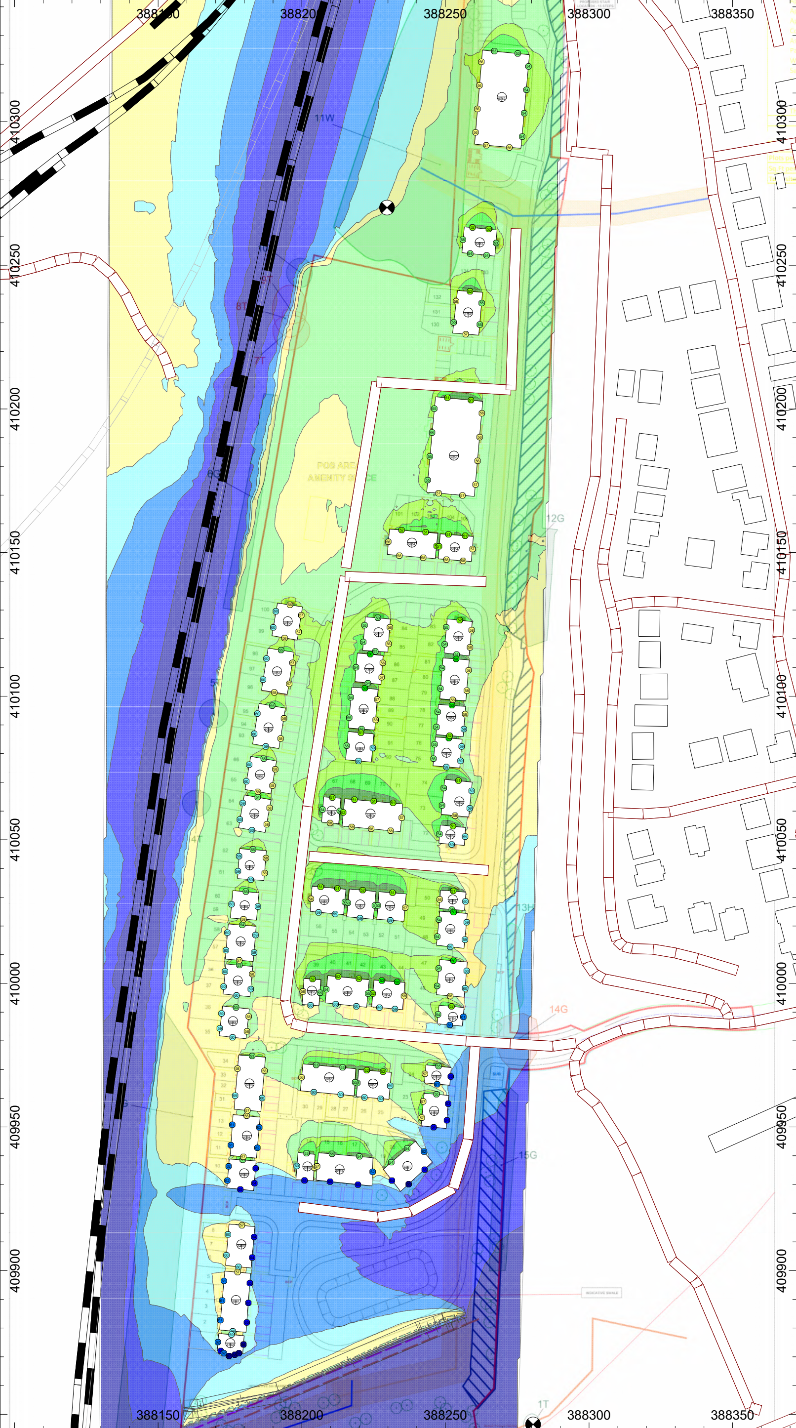
Figure 3 - Daytime Grid Noise Map (BS 8233) - Calculation at 1.5 m above ground level
