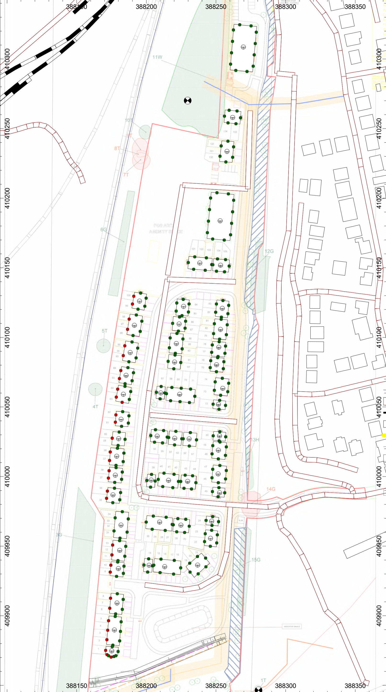
Figure 5 - Night-time Maximum Noise Level Grid Noise Map (WHO) - Calculation at 4 m above ground level
