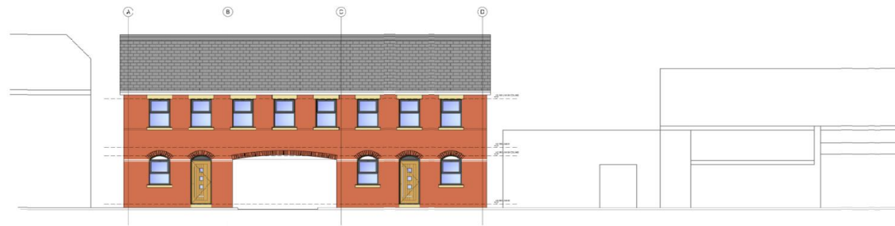
SOUTH FACING (BOARSHAW ROAD) ELEVATION 1:100
