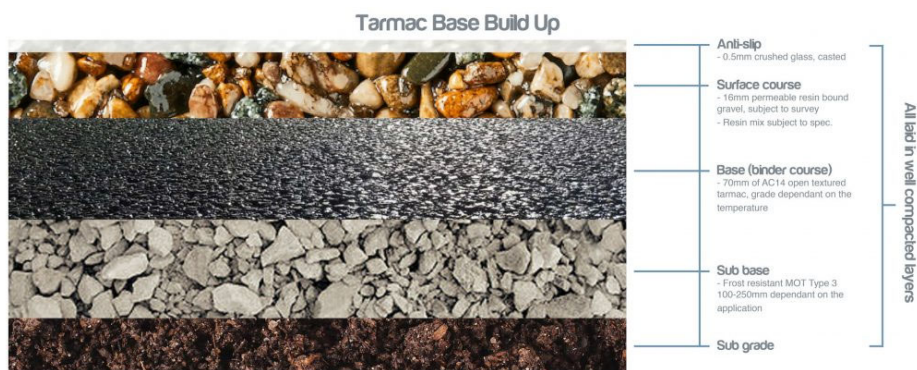
Free Draining Permeable Resin Bound Parking Bays.
