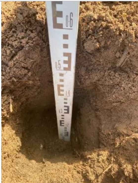
Depth of Cover System at Ground Level
