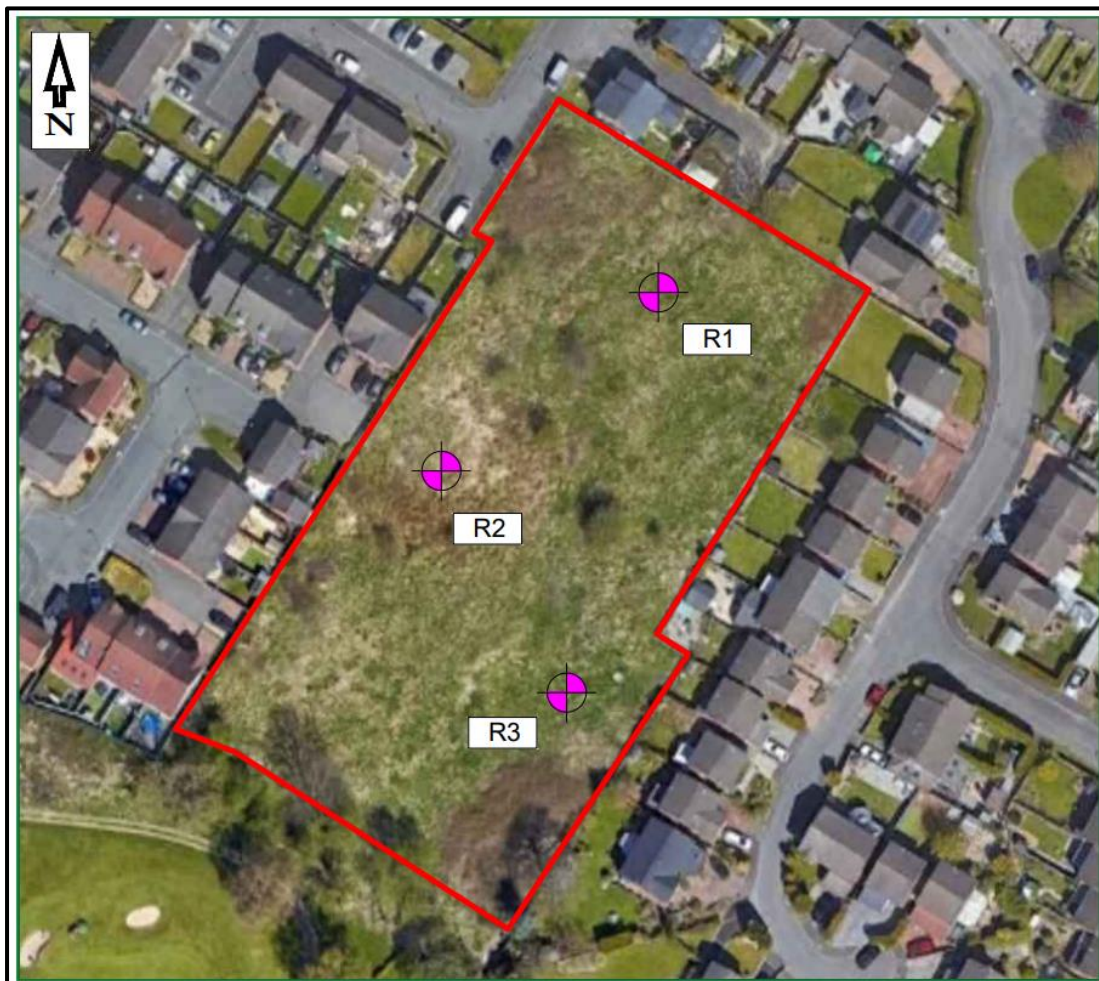
Figure 4: Rotary Borehole Locations
