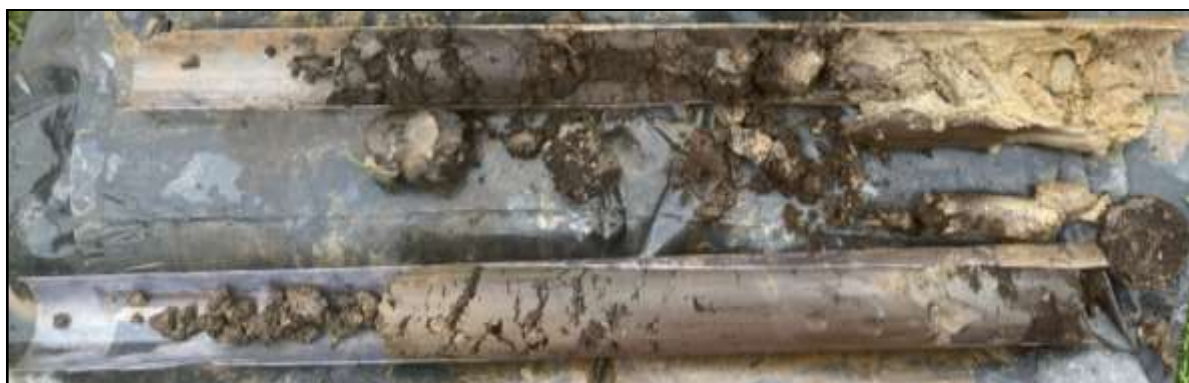
Figure 7-3: A photograph of the Peat observed from WS01 from 1.0m – 2.0m depth
