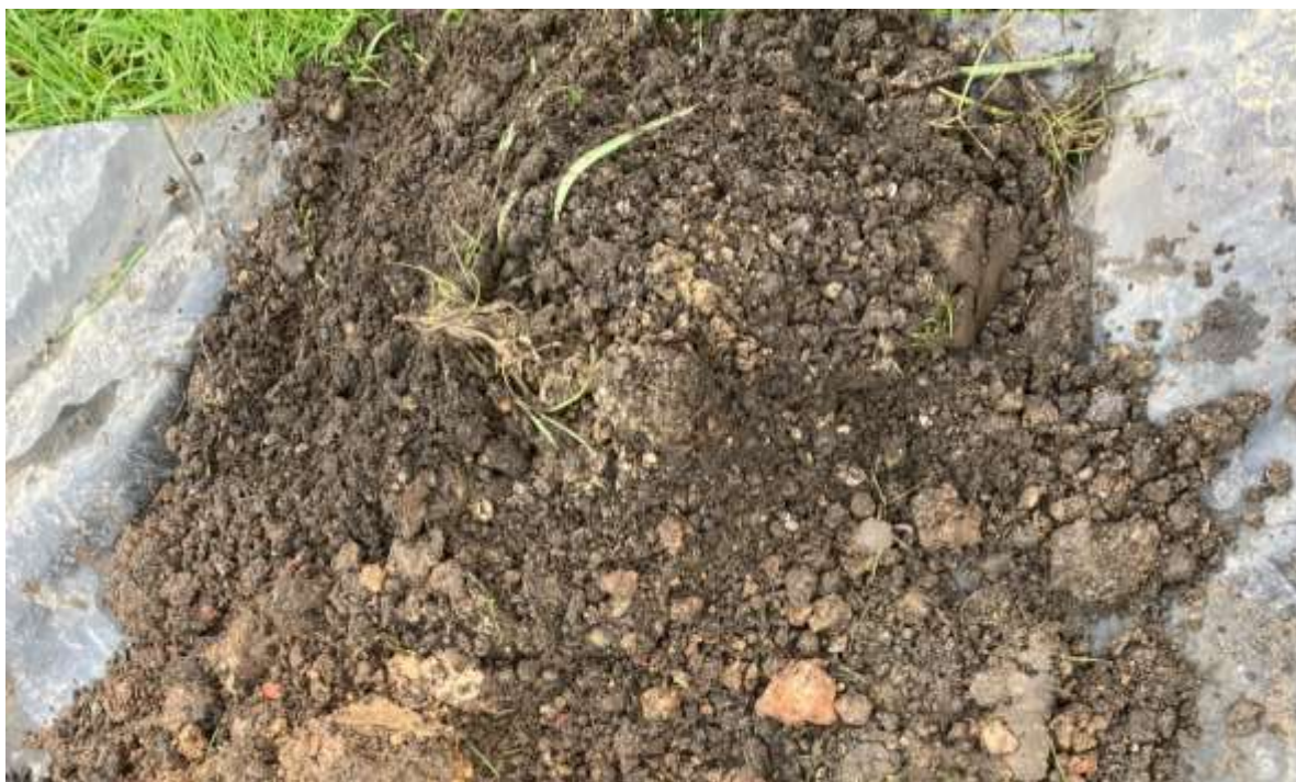
Figure 7-1: A photograph of the Made Ground from WS01 0.30m – 0.80m
