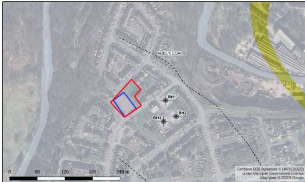
Figure 2-10: Location of GRM Development Solutions boreholes in relation to the site and the Arley Coal seam
