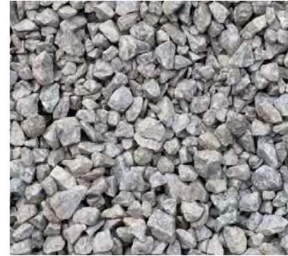
Loose limestone / hardcore chippings
