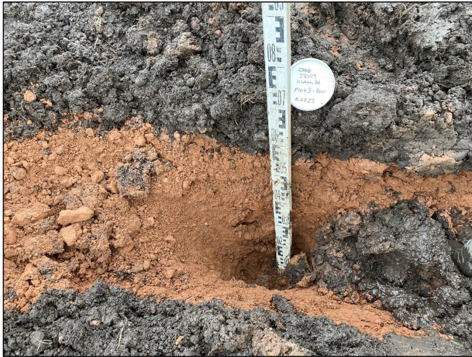
View of Plot 3 rear garden excavated to a depth of 0.75m.
