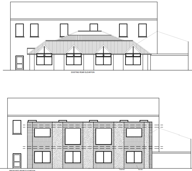
Figure 3: Existing/Proposed Rear Elevations Plan Extracts (NASA Design Studio), NTS
