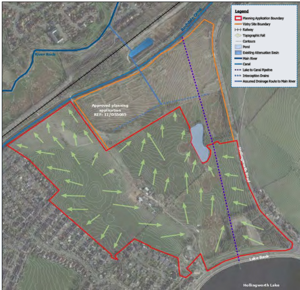
Figure 3: Existing Drainage Plan (Betts Hydro, 2022)
