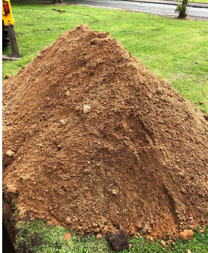
PLATE 3 GRAVELLY SAND MATERIAL – TP103
