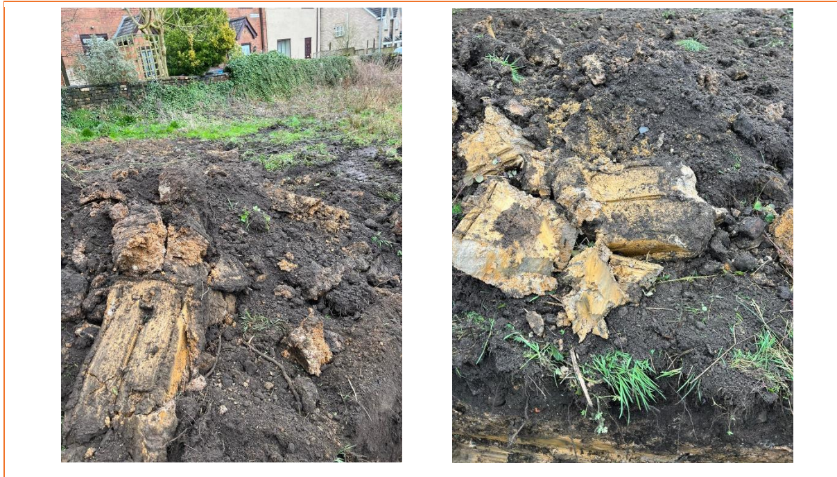
FIGURE 1.2 PHOTOGRAPH OF THE SPOIL FROM TRIAL TRENCHES INDICATING NATURAL SOILS
