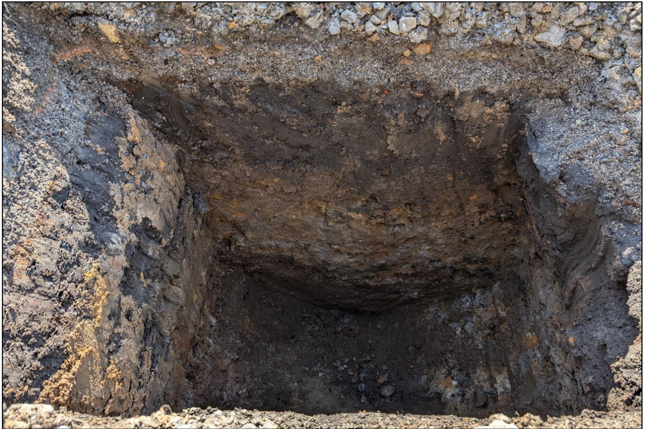
Infiltration Test Hole 1/Front of Site/Arnside Rd.
