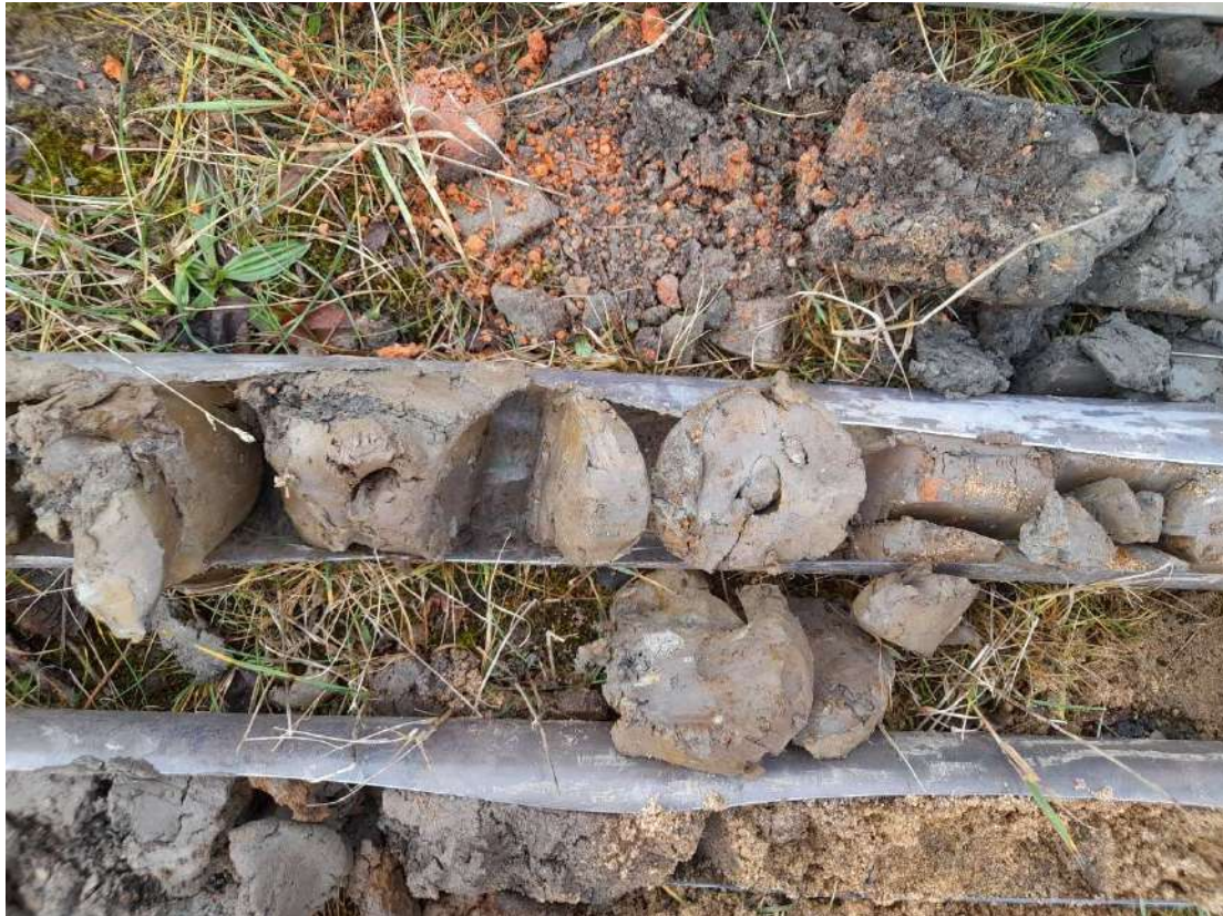
Borehole WS2, showing close-up of glacial clay.
