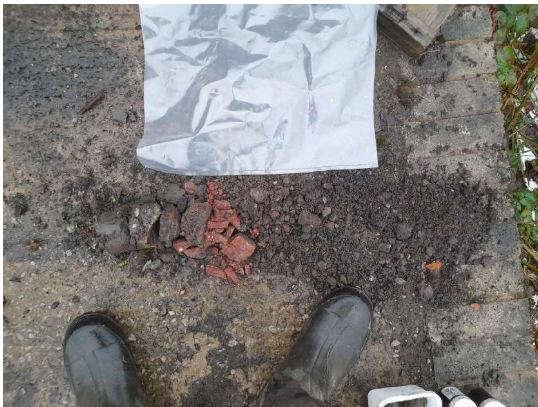
Borehole WS6 a-c typical soil arisings.
