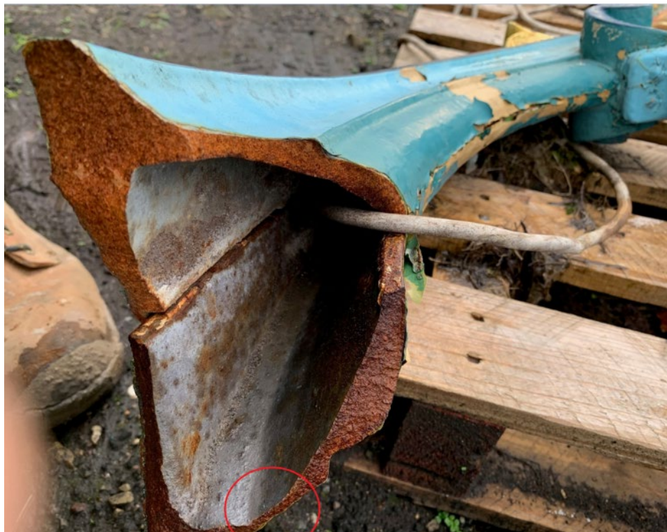
Thin section to Lighting Arm
