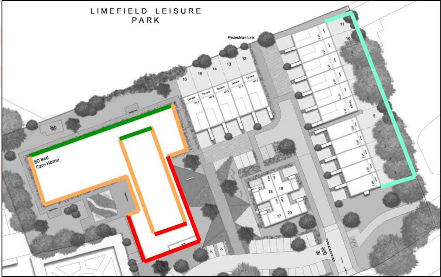
Figure 1: Care home façade treatment mark-up (red, orange, green) and noise barrier location (cyan)
