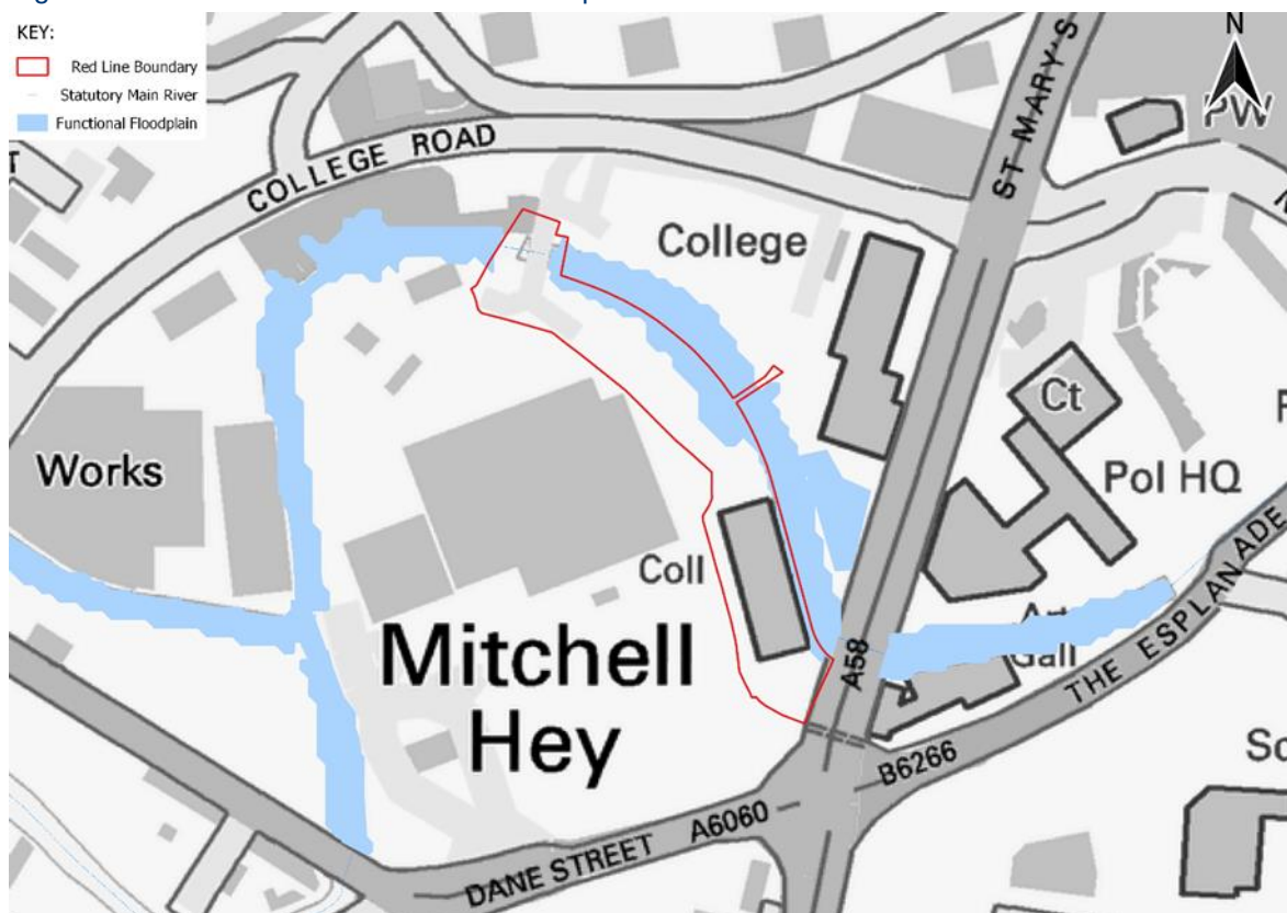
Figure 4: Definition of the Functional Floodplain
