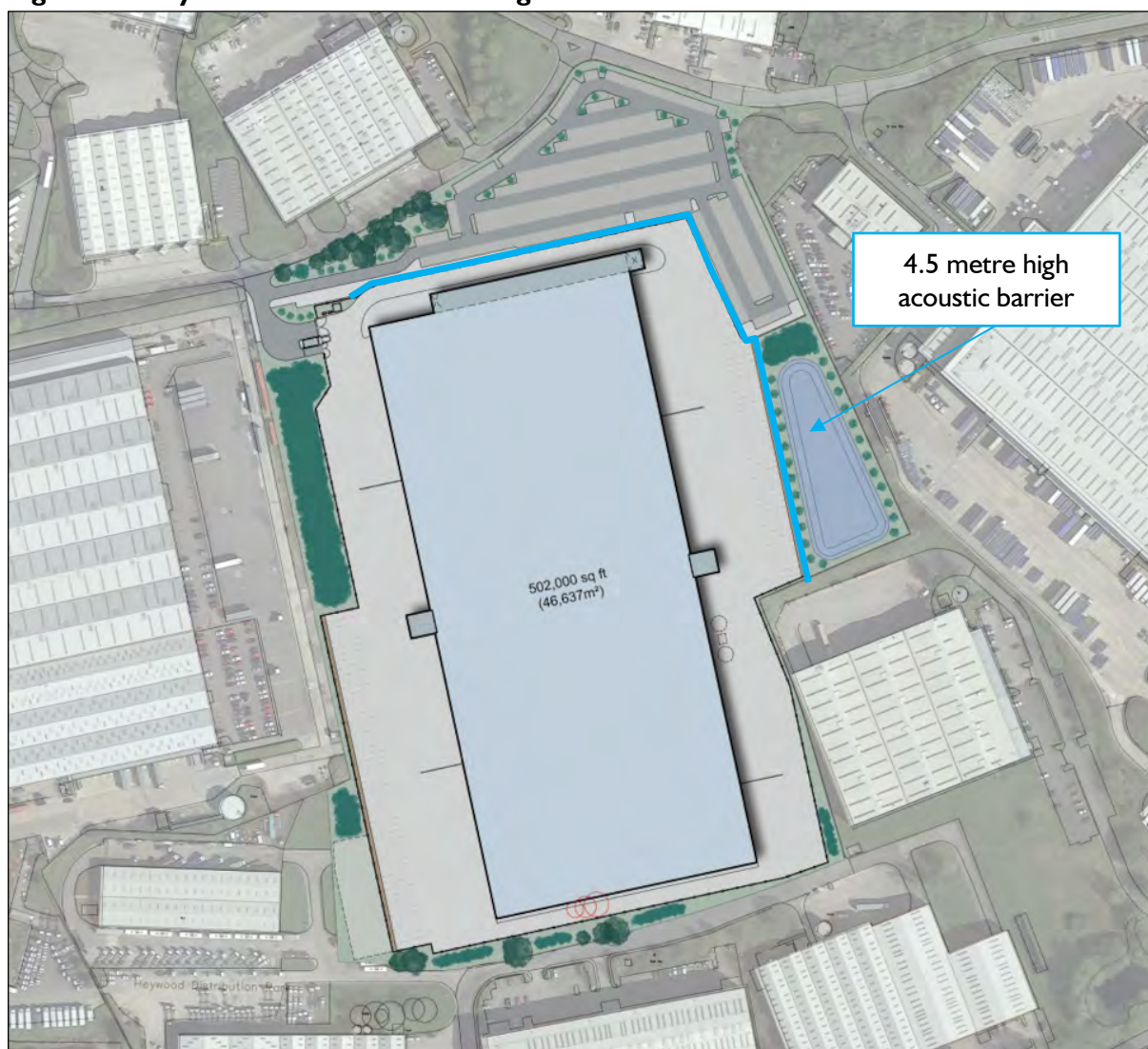
Figure F.2: Layout I - acoustic barrier alignment
