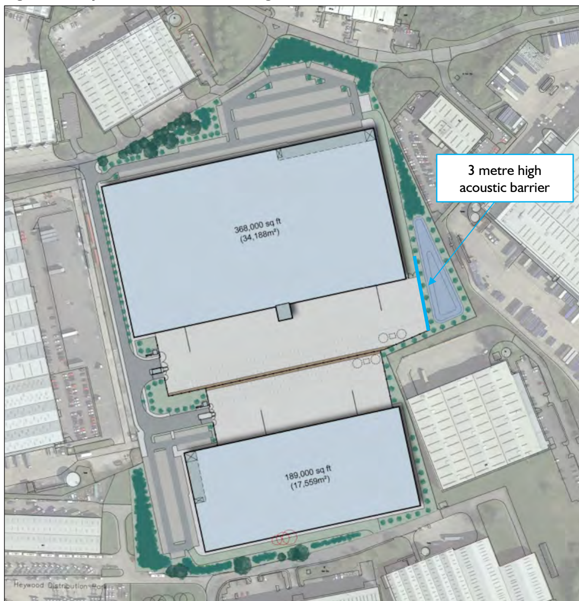
Figure F.3: Layout 2 - acoustic barrier alignment
